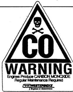
**A WARNING DECAL is provided by WESTERBEKE and should be fixed to a bulkhead near your engine or generator. WESTERBEKE also recommends installing CARBON MONOXIDE DETECTORS in the living/sleeping quarters of your vessel. They are inexpensive and easily obtainable at your local marine store.**
